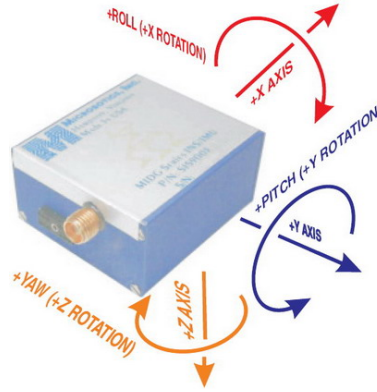
Figure 6.6: Inertial navigation system (INS) aided with GPS (MIDG II), the equipment shown with its sensors sensitive axes ( Microbotic, Inc. )
