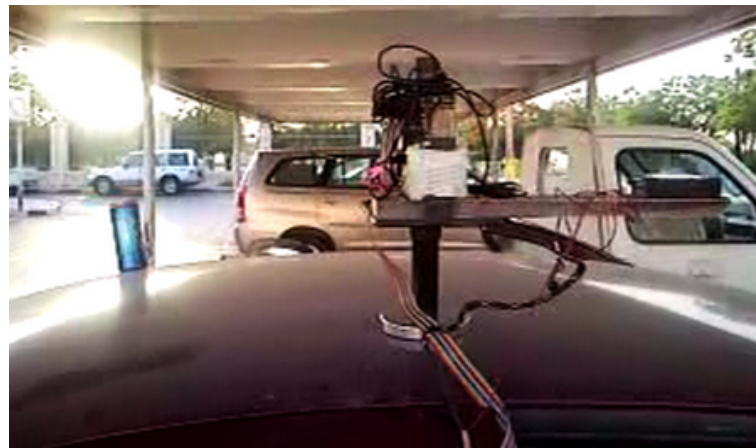
Figure 6.18: A view of INS/GPS navigation setup fixed on vehicle's roof as close as possible to the center, since the vehicle is considered as a small size vehicle, then the lever arm between the location of the setup and the center of the vehicle gravity is neglected.
