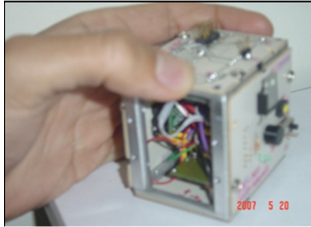
Figure 3.2: Constructed (6-DOF) IMU unit, which consists mainly from triad of gyros and accelerometers sensors. The unit dimensions are (5.9 \times 4.6 \times 5.8) cm.
